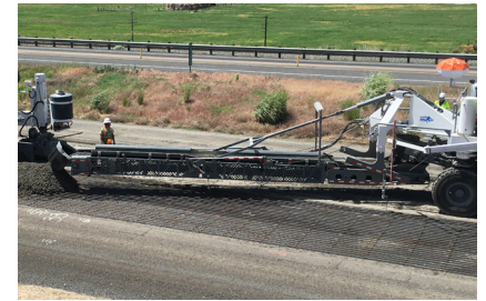
Hinging Swing Conveyor. 35 ft. (10.66 m) Long with 170° Swing Capability
