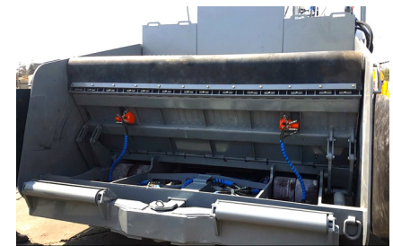
Hinge Up Flop Gate with Shuttle Plate
